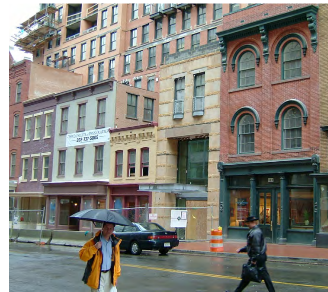
Larger-scale buildings can be successfully incorporated into lower-scale historic areas with the use of upper-level setbacks and contextual design.
