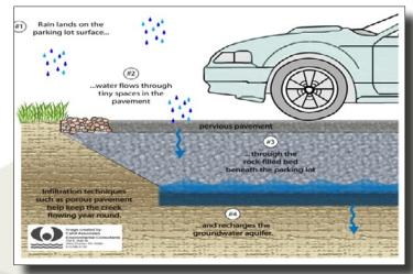
• Have your pervious pavement professionally maintained annually. A vacuum truck or a specialized sweeper can clear out the pores that have filled in over time.
