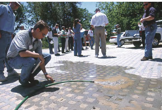
Permeable paving demonstration
