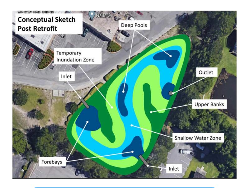
One wet pond in the University Commons complex is proposed to be converted into a stormwater wetland to improve pollution treatment capabilities and increase habitat in the area. Above is a conceptual sketch of the wetland design.
