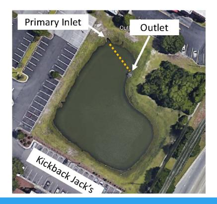
The Sam's Club wet pond is currently designed with a very short stormwater residence time, meaning that stormwater can essentially flow from the inlet to the outlet without treatment.
