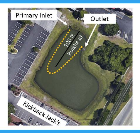
A baffle is proposed to increase the residence time of stormwater in the pond, which will increase the amount of pollution that can be settled out before reaching the outlet.
